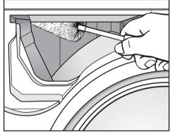
Use a bottle brush to remove detergent residues and limescale from the jets inside the detergent dispenser drawer housing.
